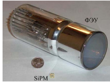
Figure 4.1 – Photo of vacuum PEM and SiPM.
